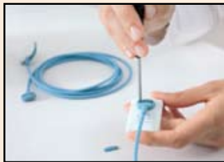
Simple cable replacement
